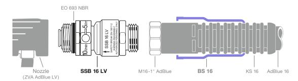
**SSB 16 LV** is a self-sealing reusable breakaway coupling with swivel for the filling of cars and transporters (Light Vehicles) with AdBlue<sup>®</sup> urea solution (DEF/AUS 32/ARLA 32). The coupling is designed to protect dispenser, hose assembly and car against damage which can occur by drive-off incidents. As a nozzle break it is fitted between **ZVA AdBlue LV** and the hose assembly. The **integrated volume flow switch** is used for calibration of the dispenser only.
